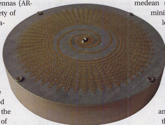
1. This photograph shows the exponential-Archimedean spiral antenna (EARSa) with highly miniaturized aperture.
